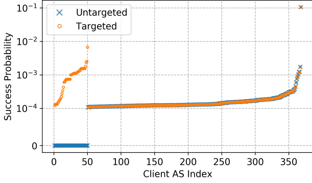
Fig. 4. Success rates of targeted attacks against DeNASA clients using 1 malicious guard relay with a bandwidth of 2,000 (0.011% of total guard bandwidth). For 86.4% client ASes, the targeted and untargeted success rates are equivalent (the overlapping points).
